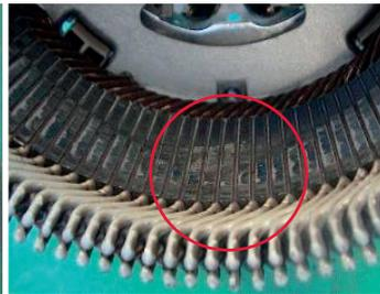
Rotor coil wire breakage
