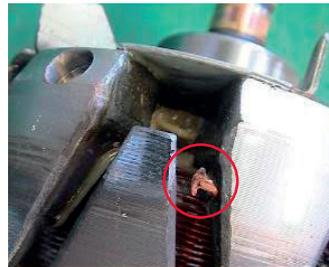
Fusing point resin crack
